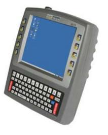
The 8515 from Psion Teklogix packs a powerful feature set in a small and lightweight frame. This small form factor Vehicle-Mount computer has exceptional functionality and provides outstanding ergonomics when considering line-of sight, safety and keyboard operation.
